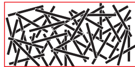
Shred Sample Size - 3.9mm x 40mm (1/8" x 1 9/16") Cross Cut Type IIIB
